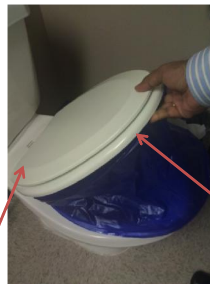
Move down the seat/lid and PlungeMAX together ensuring that the bottom of the PlungeMAX stays in place to make a Plunge The base of the PlungeMAX will rest on the seat rim sealing it and compressed air escaping through the bottom three holes into the toilet bowl (This is the critical part – if the bottom of the PlungeMAX shifts during this action – the seal will be compromised and the air will escape without plunging)
