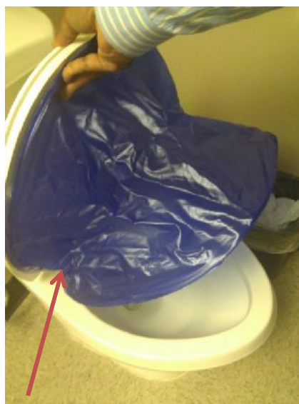
Move down the seat/lid and PlungeMAX together ensuring that the bottom of the PlungeMAX stays in place to make a Plunge The base of the PlungeMAX will rest on the seat rim sealing it and compressed air escaping through the bottom three holes into the toilet bowl (This is the critical part – if the bottom of the PlungeMAX shifts during this action – the seal will be compromised and the air will escape without plunging)
